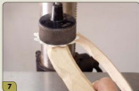
7 Shaping the outside edge of the ripple. Use the hook-and-loop pad sander with a coarse grit to shape and smooth the outside of the ripple.
