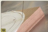
12 Cutting the outside box body. Using repositionable adhesive, attach the box body pattern to the 3/4" (22mm)-thick piece of cherry. Drill a straight entry hole near a corner in each segment with the 1/8" (3mm) drill bit. Tilt the saw table to 15°, left side down, and cut clockwise around the outer circle.
