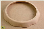
10 Rounding over the edges. Round over the underside of the lower outer edge.
