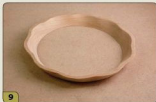
9 Completing the sanding. Using both sanders, sand with increasingly finer grits until the rim is well-shaped and smooth. Soften the upper edges.
