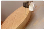
Cutting clockwise with the saw table tilted left side down creates a cut that is wider at the top of the wood than the bottom.
