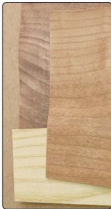
Veneer. Veneer can add the same effect as thin sheets of contrasting wood, but at far less cost.
