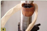
8 Shaping the inside edge of the ripple. Use the inflatable ball sander with a coarse grit to shape the inside of the ripple until the curves are smooth.
