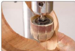
Inflatable round sanders are necessary to sand the inside of rings, flutes, and other concave surfaces.
