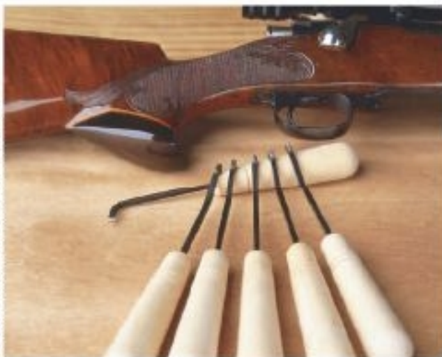
Checkering tools can be used to create a repeating grid pattern on a gunstock. Some carvers find that file-like checkering tools are an excellent choice for the fine detailed carving of fur, hair, and feathers.
