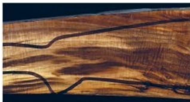
A gunstock blank pattern placed on three different species of myrtle shows how varied wood can be. Top to bottom: tiger myrtle, dark myrtle, and myrtle (grain affected by a knot).
