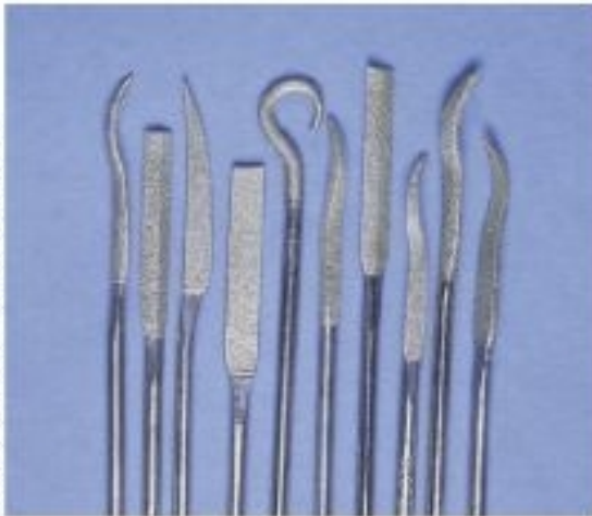
Files are available in fine grit, like this 10-piece set, and coarse grit and are handy for removing wood in small areas of relief carving.
