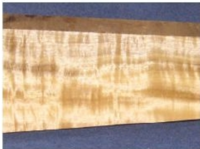
A windowpane myrtle wood blank is ready to be marked up for band sawing.
