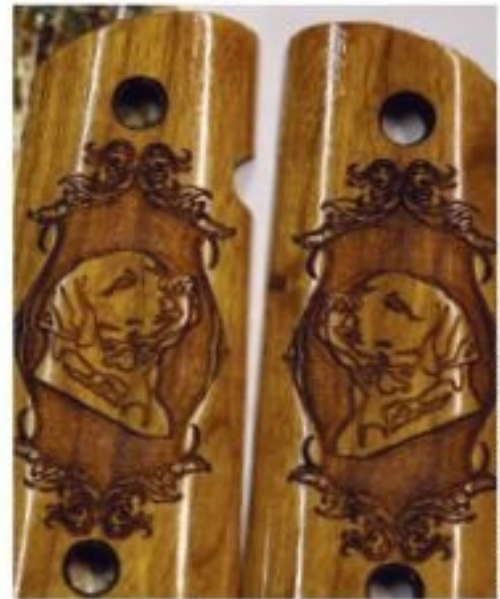
Patterns can be taken to a laser engraver for a delicate, low relief reproduction of personalized artwork. This image was created from a photograph, but any shaded pattern will also work well.
